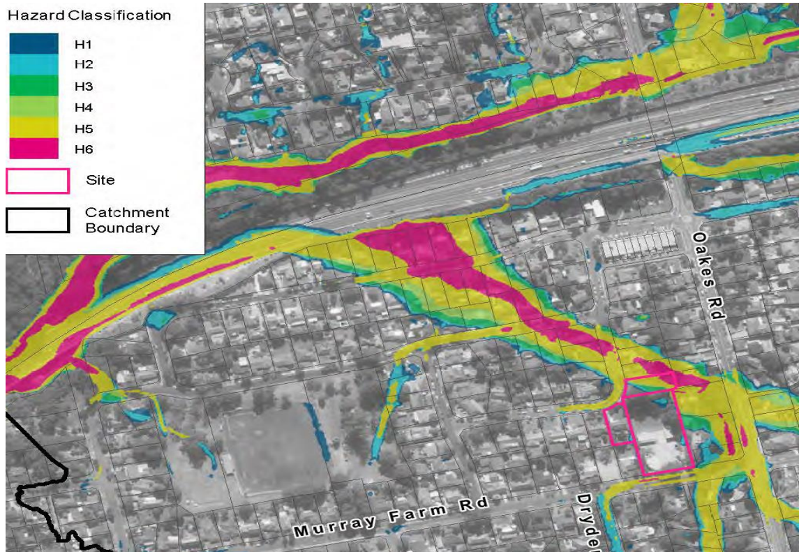
Figure 12: PMF Flood Hazard Classification model, Source BMT
